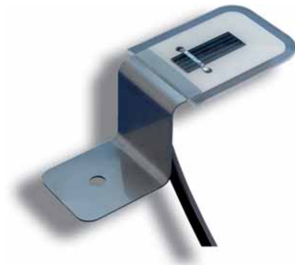
Spektron 210: The 2-core extension cable is UV-resistant. All Spektron devices are calibrated beneath a sun light simulator against a reference sensor, which has been calibrated by the Fraunhofer ISE.
