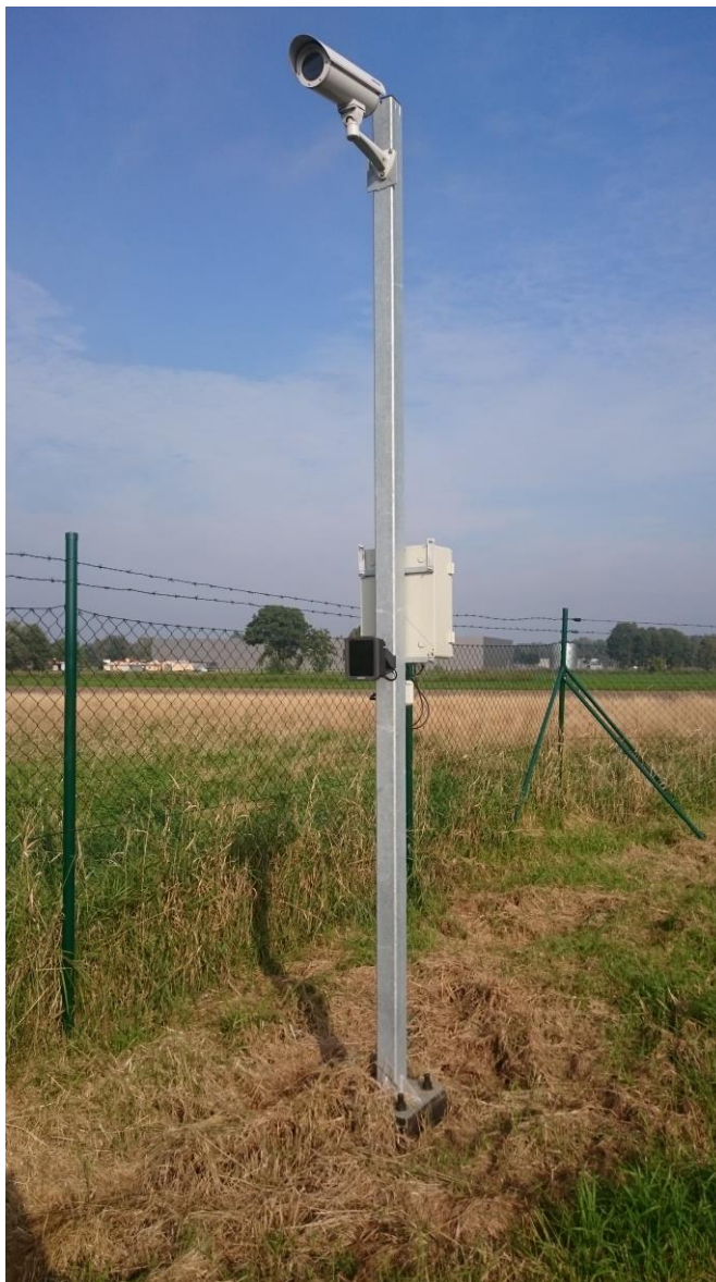
Image 60: CCTV camera and AC3CON mounted on a pole. We can observe specific IR lamp mounted below the camera to help get better image of the camera during the night. [own photo]
