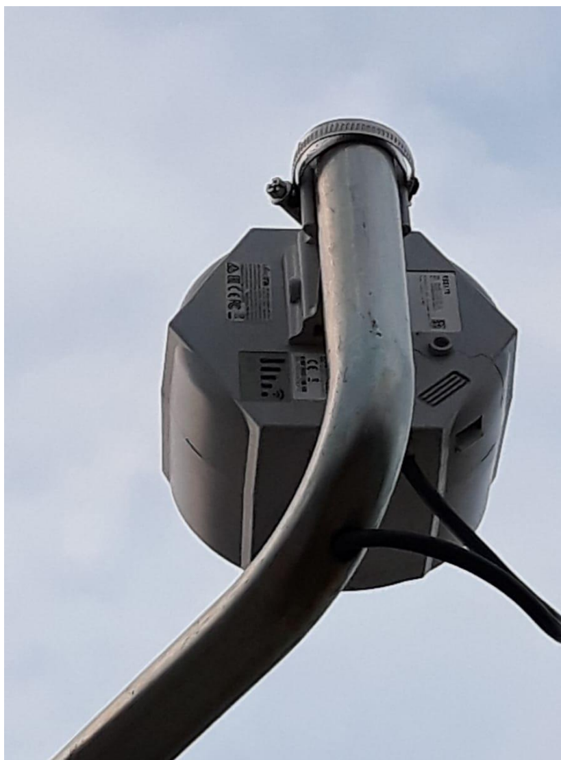
Image 78: 10-dBi directive Mikrotik antenna to increase. [own photo]
