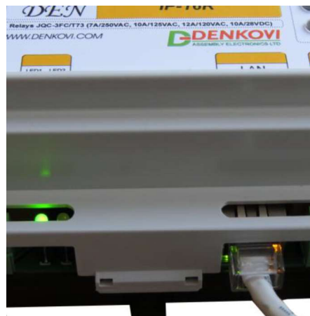
Figure 7. Connecting a LAN cable
