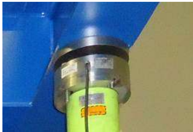
Figure 4. Detail of the load cells.
