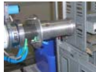
Fig. 6. PA-10 with an electrical screwdriver.
