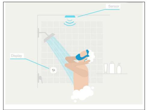
Fig.3. Location of the Display and the Sensor in the shower cabin. Source: Aguardio ApS
