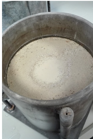
Figure 17: Sample after submerged penetration.
