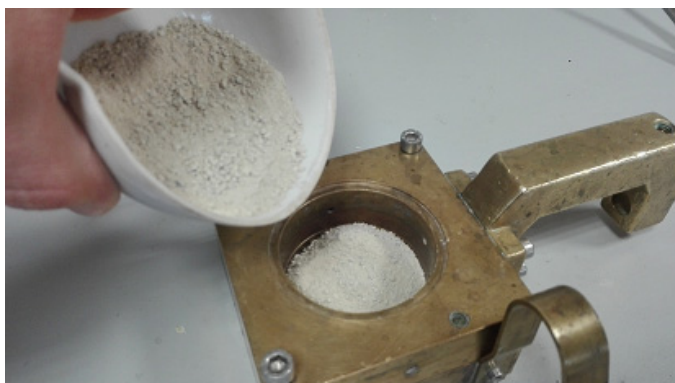
Figure 2: Pouring the sand into the box.
