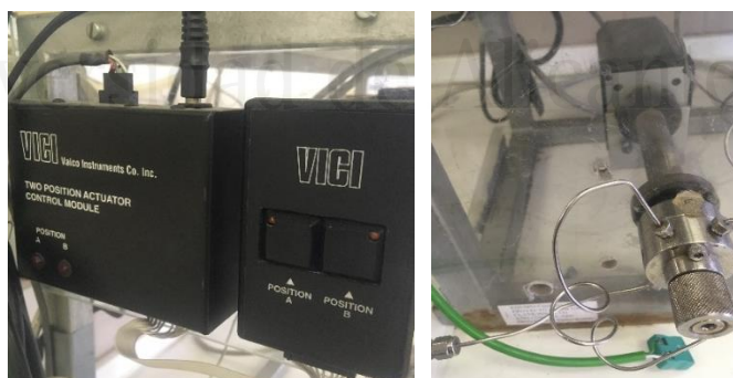
Figure 2.12. (Left) Control module actuator of the two-position high precision injection valve. (Right) injection valve with loop.
