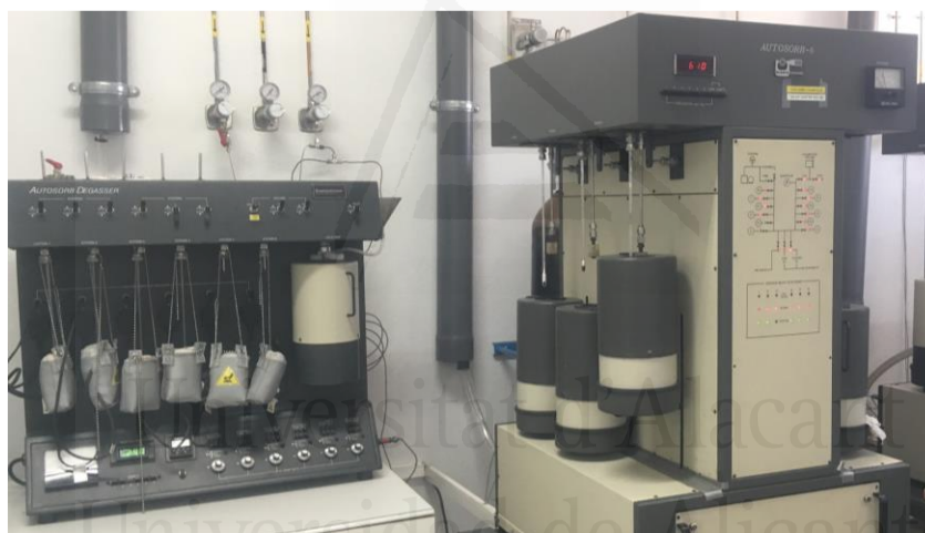
Figure 2.1. Degasification (left) and adsorption (right, Quantachrome Autosorb-6B) instruments to record \text{N}_2 adsorption isotherms -196^\circ\text{C} .
