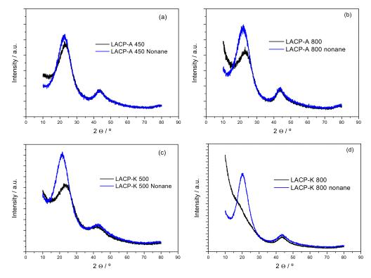
**Figure 4.** XRD profiles for the peach stone-based activated carbon after (**a**, **b**) acid (LACP-A) and (**c**, **d**) KOH (LACP-K) activation prepared at (**a**, **c**) low and (**b**, **d**) high activation temperature, and before and after incorporation of different hydrocarbons.
