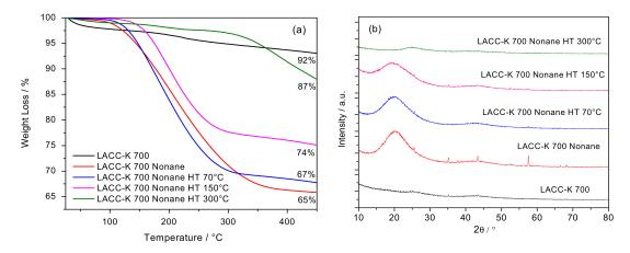
**Figure 2.** (a) Thermogravimetric analysis of sample LACC-K 700 before and after exposure to n-nonane, and LACC-K 700 sample after different thermal treatments under inert atmosphere; (b) XRD pattern for the samples evaluated.
