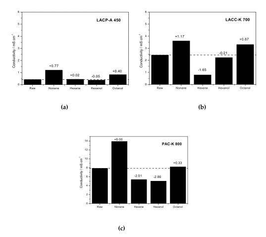
**Figure 6.** Electrical conductivity (mS/cm) measured for the three activated carbons: (**a**) LACP-A 450; (**b**) LACC-K 700 and (**c**) PAC-K 800, evaluated before (raw) and after adsorption of different hydrocarbons or alcohols (nonane, hexane, hexanol and octanol).
