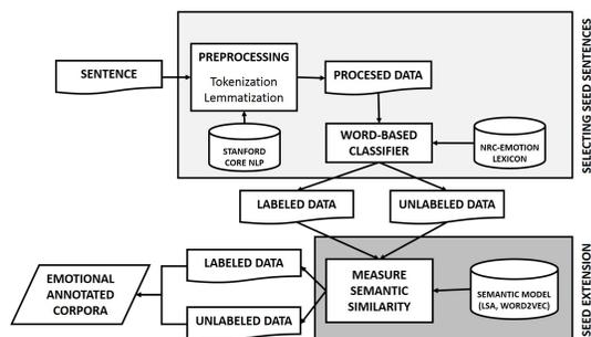
Fig. 1. Overview of the initial categorization step (Step 1 of bootstrapping).
