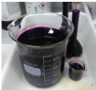
Figure 3.16: glassware kept in a permanganate solution.
