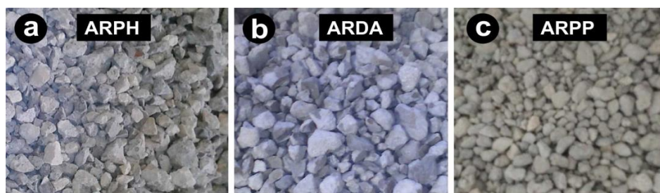
Figure 1. Recycled aggregates (RA) from three sources used as a coarse aggregate in hot asphalt concrete. (a) Obtained by crushing concrete specimens; (b) from demolition of Havana sidewalk and (c) from precast plant waste.
