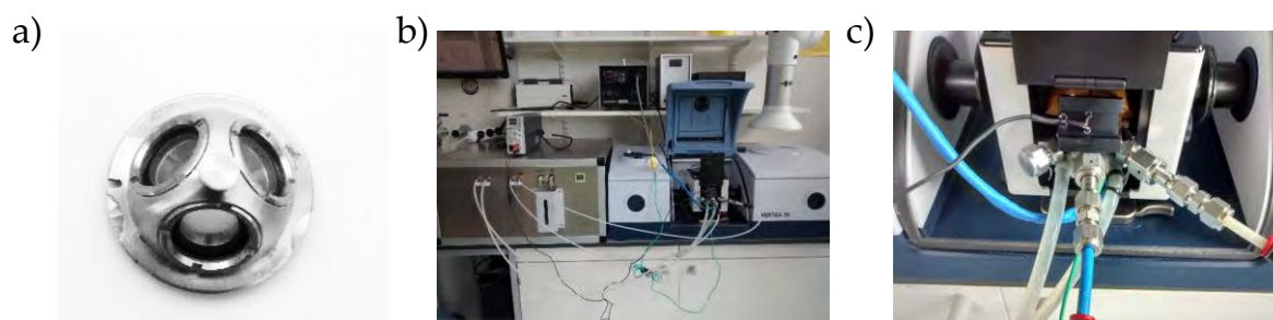
Figure 7.1. Images of the FTIR device used: a) Three-window cell, b) In situ DRIFT setup and c) detail of the analysis chamber.
