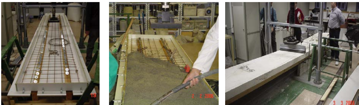
Figure 9: Production of full-scale prototypes and testing of prototype in elastic range and until failure.
