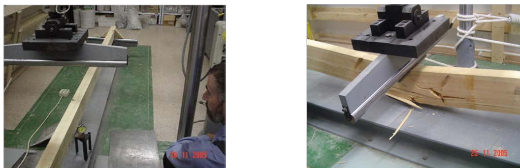
Figure 7: Wood bending tests in elastic range and at breakage.
