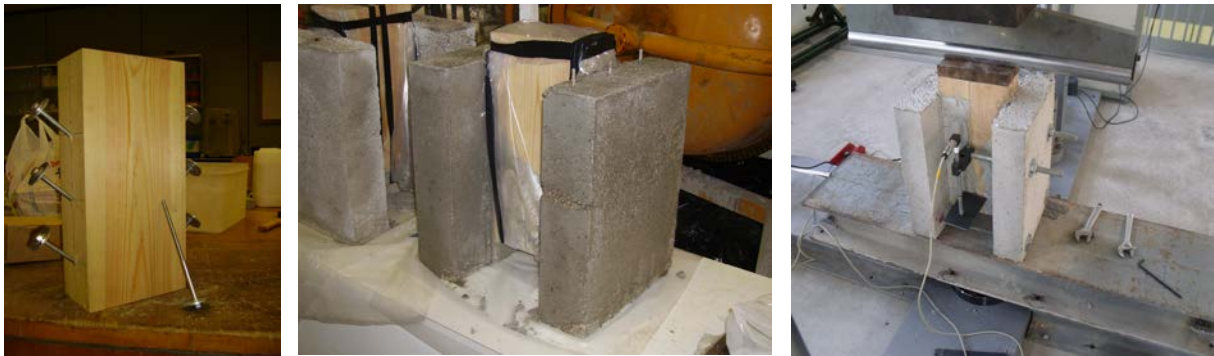
Figure 8: Manufacturing steps of a specimen connection and push-out test.
