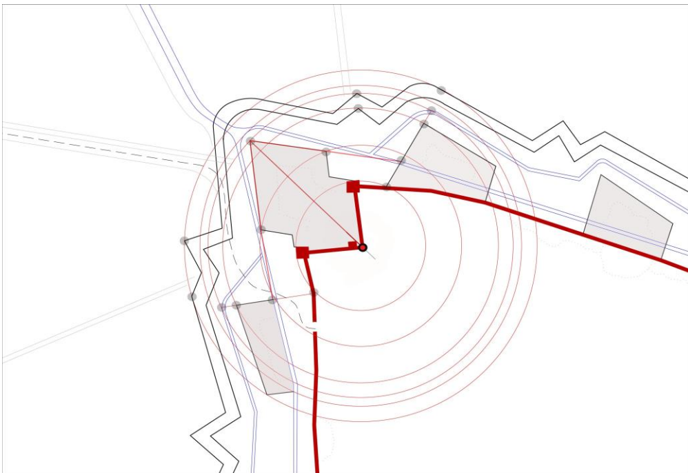
Fig. 7- Graphic construction of the north-west sector of the seventeenth-century front. There is a close link between the pre-existing structures - which guides the design setting - and the new "necessities" that are functional to the "modern" defense of the city
