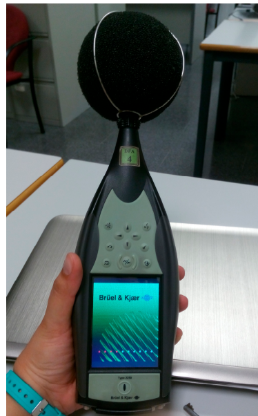
Figure 11. A Bruël & Kjaer Type 2250 sound level meter.
