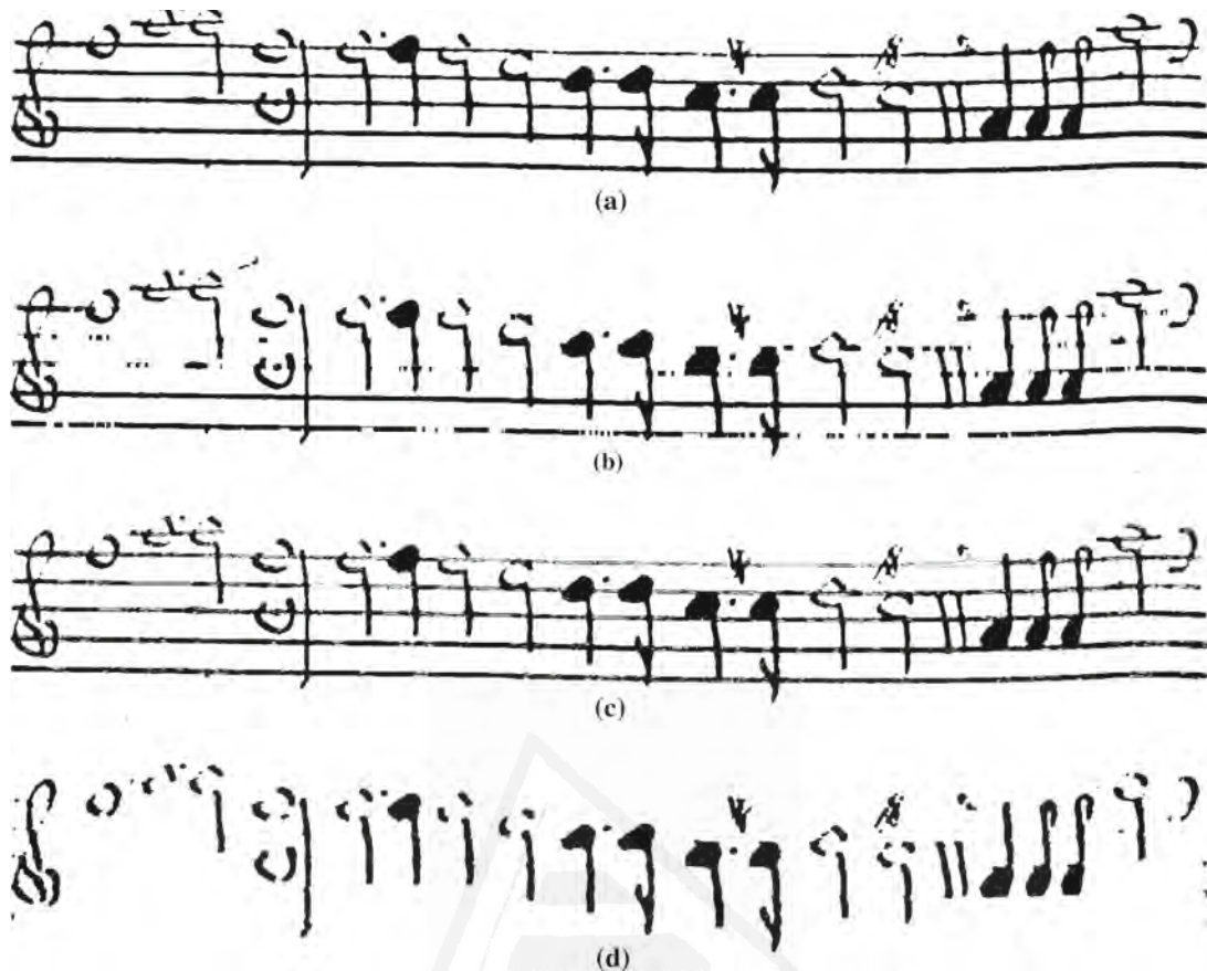
Fig. 8 Performance of LRDE method and our proposal (SVM classifier and 81 features per pixel) with general and specific data over an ancient score of early music. a Input score. b Input score after staff
