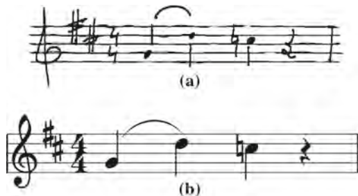
Fig. 1 The task of optical music recognition (OMR) is to analyse an image containing a music score to export its musical content to some machine-readable format. a Example of input score for an OMR system. b Symbolic representation of the input score
