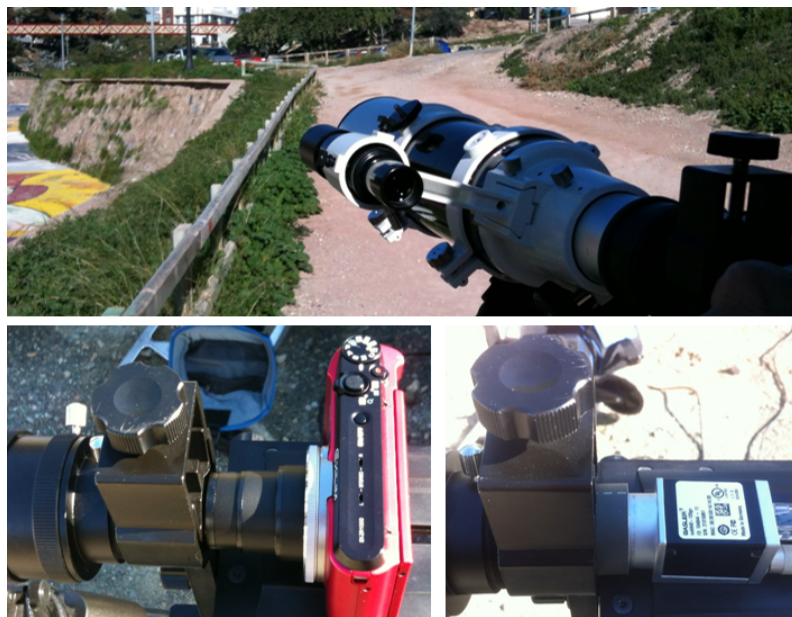
Fig. 3 General view of the set up recording at 200 m (upper side); detail of the connection between Casio camera and telescope (lower and left side); detail of the connection between Basler camera and telescope (lower and right side)
