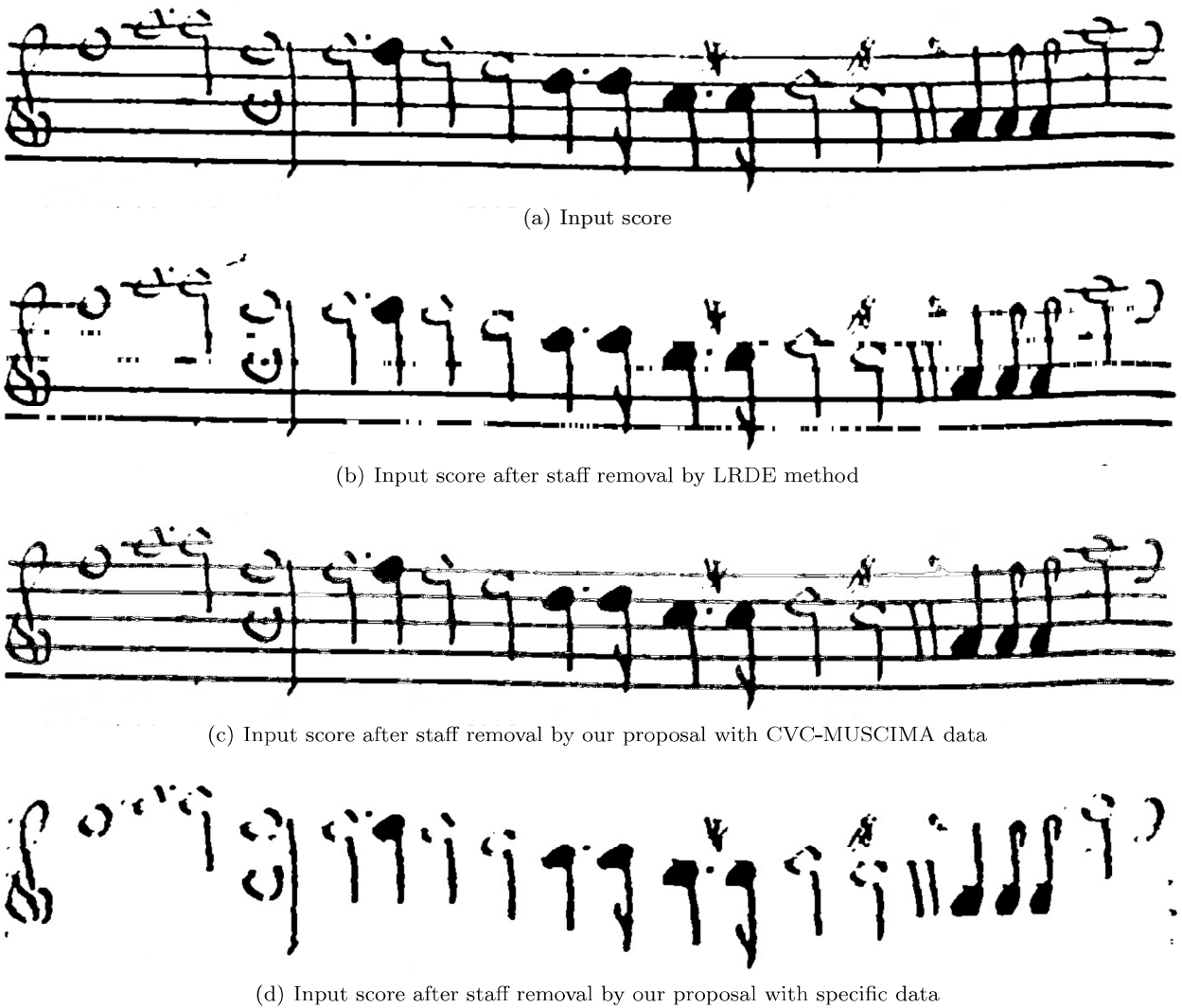
Fig. 8 Performance of LRDE method and our proposal (SVM classifier and 81 features per pixel) with general and specific data over an ancient score of early music.
