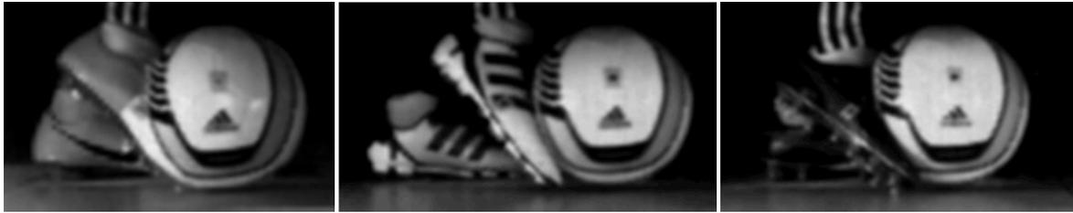
Figure 3. Ball deformation during impact for boot A, B and C
