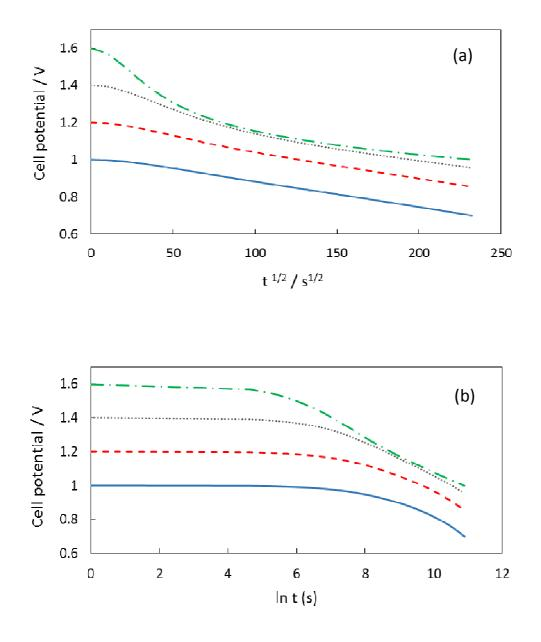
**Figure 6.** Cell potential (–), positive electrode potential (–), negative electrode potential (–) *vs* time for an AC-PTFE/AC-PTFE capacitor with reference electrode in 2.0 mol L<sup>-1</sup> lithium sulfate after 3 h of potential hold at  $U_i = 1.0$  and 1.4 V. Temperature  $24 \pm 1^{\circ}$ C.
