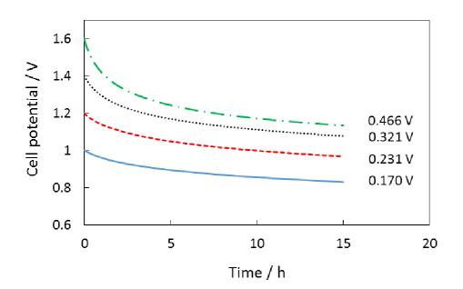
**Figure 2.** Leakage current of an AC-PTFE/AC-PTFE coin-cell capacitor in 2.0 mol L<sup>-1</sup> Li<sub>2</sub>SO<sub>4</sub> vs floating time for various values of potential hold U<sub>i</sub> = 1.0 V (-), 1.2 V (- -), 1.4 V (···) and 1.6 V (- · -). Temperature  $24 \pm 1^{\circ}$ C.
