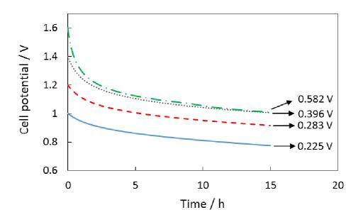
**Figure 4.** Leakage current of a AC-PTFE/AC-PTFE coin-cell capacitor in 2.0 mol L<sup>-1</sup> Li<sub>2</sub>SO<sub>4</sub> vs floating time for various values of potential hold U<sub>i</sub> = 1.0 V (-), 1.2 V (- - -), 1.4 V (···) and 1.6 V ( - · - ). Temperature  $34 \pm 1^{\circ}$ C.
