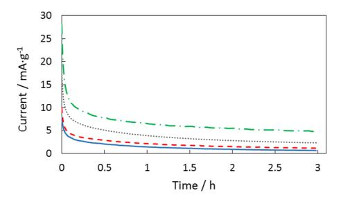
**Figure 3.** Self-discharge profiles (U *vs* t) of a AC-PTFE/AC-PTFE coin-cell capacitor in 2.0 mol L<sup>-1</sup> Li<sub>2</sub>SO<sub>4</sub> after 3 h potential hold at  $U_i = 1.0 \text{ V}$  (--), 1.2 V (- - -), 1.4 V (···) and 1.6 - (- ). Temperature  $34 \pm 1^{\circ}$ C. The value of cell potential drop after 15 hours is indicated close to each curve.
