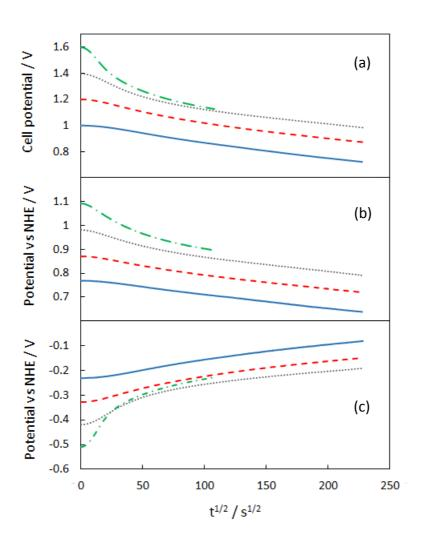
**Figure 8.** (a) Cell potential, (b) positive electrode potential, (c) negative electrode potential *vs* ln t for an AC-PTFE/AC-PTFE capacitor with reference electrode in 2.0 mol L<sup>-1</sup> lithium sulfate after 3 h of potential hold at  $U_i = 1.0$  (--), 1.2 V (- - -), 1.4 (···), and 1.6 V ( - - ). Temperature  $24 \pm 1^{\circ}$ C.
