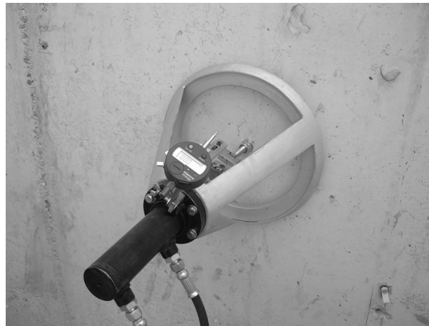
Figure 2. Test pullout (anchorage-resistant element).
