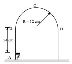
**9.-** A small object rolls without friction around the track shown in the figure. It starts from the rest at a point at a height h above the bottom of the loop. What is the minimum value of h (in terms of R) such as the object moves around the loop without falling off at the top of the vertical circumference of radius R.
