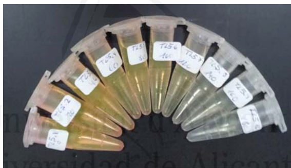
Figure 4.11. Photographs of the different samples taken along the degradation reaction of an aqueous solution of R6G ( 5 \cdot 10^{-5} M) under UV radiation using \text{TiO}_2 -PPD-b as photocatalysts.
