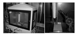
FIGURE 3. The left figure shows the apparatus used to determine sample flammability using the single flame test. The right figure shows the burner utilized in the test along with the vertically-placed test sample.
