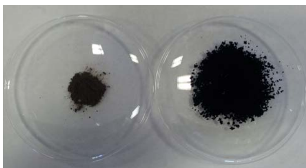
Figure 6. Digital images showing the increase in volume after blasting and the colour change from brown to black as a consequence of the thermal reduction. GO (left) and TRG127 (right).
