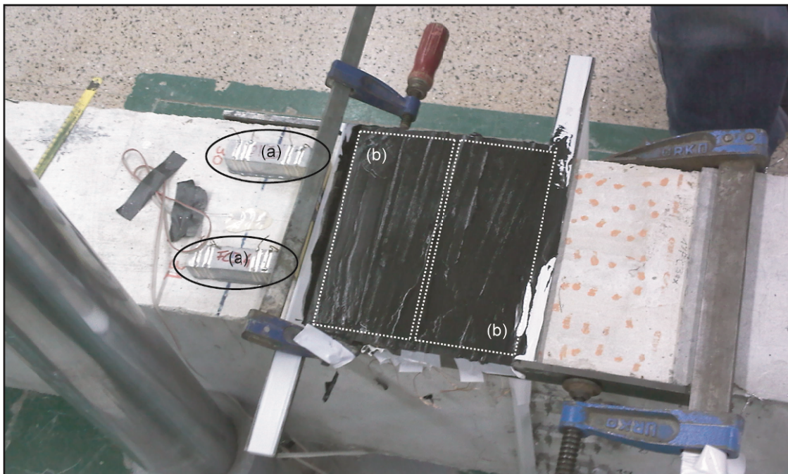
Figure 7. Class of sensor according to its dimensions: (a) 2 \times 2 \times 8 \text{ cm}^3 ; (b) 0.7 \times 20 \times 8 \text{ cm}^3 .
