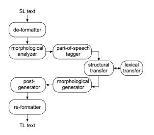
Figure 1: Modules of the Apertium shallow-transfer MT platform (see section 2).
