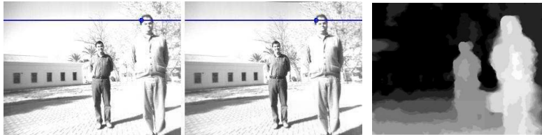
Figure 3.1: A stereo pair showing an epipolar line (left). Image of disparity (right)
