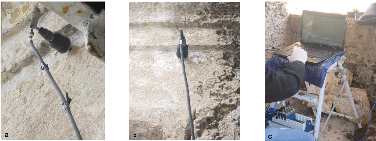
Fig. (5). Accelerometer n°2 (a), Accelerometer n°4 (b), Instrumental system (c).
