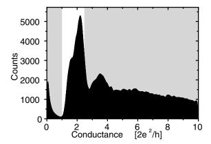
FIG. 3. Histogram of the number of times each conductance value is obtained for a large number ( $\sim 2000$ ) of individual digitized conductance traces similar to the one shown in Fig. 1, recorded while repeatedly breaking the Pt contact. The high-lighted area indicates the range between the  $G_{\text{start}}$  and  $G_{\text{stop}}$  value used to define the length of the last plateau when recording the length-histogram in Fig. 2.
