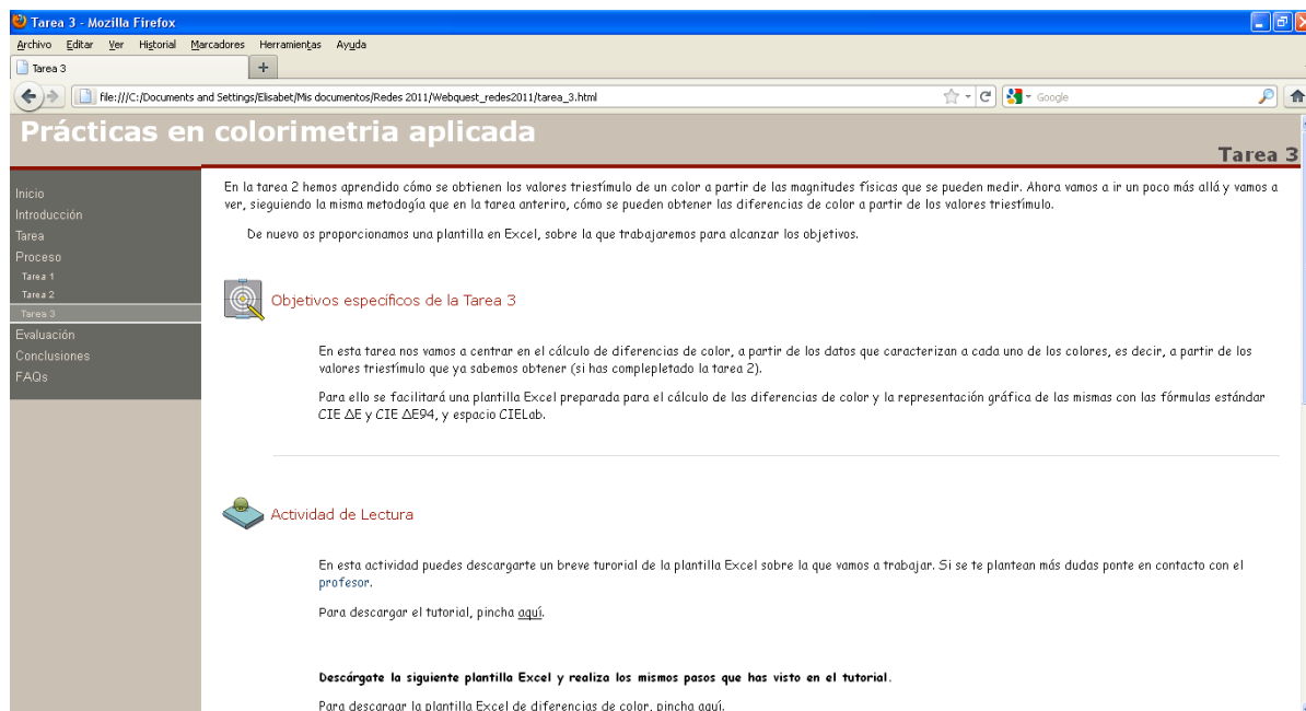
Fig.3. Task 3: computation of colour differences by using an Excel template. The calculations in the Excel file, after doing the activity 2, allow to the abstraction. The student is focused on understand the concepts by avoiding the difficult calculations with a manual calculator.
