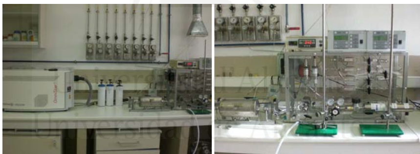
Figure 12. Quartz microreactor connected to a mass spectrometer for pulse experiments with isotopic gases.
