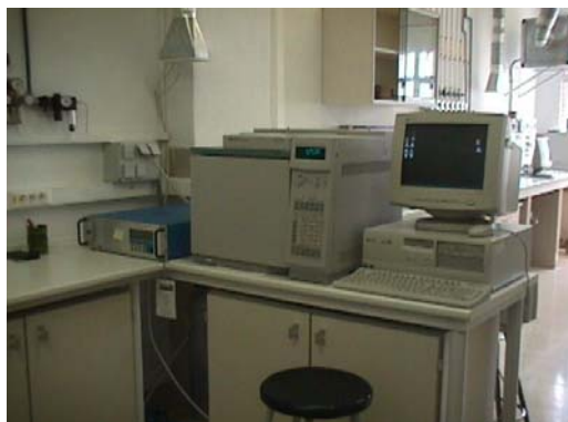
Figure 11. Gas analysis system: Gas chromatograph + NO x chemiluminescence analyzer.
