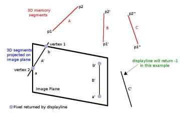
Fig. 3. Segments projection onto the image plane
