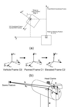
Fig. 6. Coordinate systems used to define the geometric model
