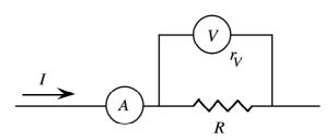
**7.-**Dynamic resistance,  $R_{din} = dV/dI$ , is a useful concept when non-ohmic circuit components are studied. For a diode, a simple model for the pn junction behaviour predicts a current-voltage relationship in the form  $I(V) = I_0[\exp(eV/kT) - 1]$ , where  $I_0$  is the saturation current, different for each diode, k is the Boltzmann's constant, T is the absolute temperature and e is the electron charge. Obtain an expression for the dynamic resistance of this device.
