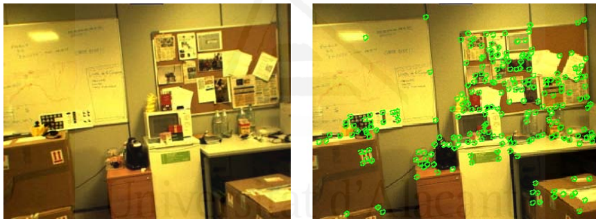
Figure 2.1: Example of Harris corners detection. Left: original image. Right: results of the Harris and Stephens algorithm.
