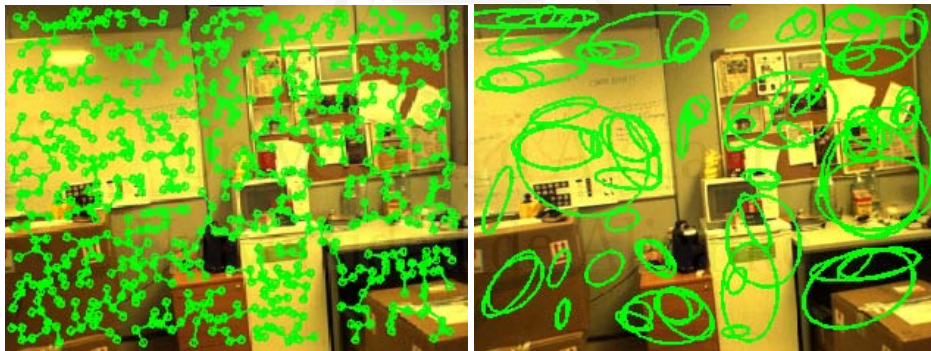
Figure 2.6: Example of application of the MSCC algorithm to the image in Fig. 2.1. Left: the MST spanning all the detected Harris interest points (represented as circles). Right: Detected regions.
