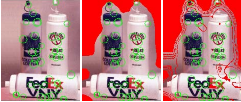
Figure 3.12: Left: output of the Scale Saliency algorithm. Center: output of the filtered Scale Saliency algorithm based on the simple test described in Section 3.3, using \sigma = 0.7 (23% of the image pixels were filtered). Right: output of the filtered Scale Saliency algorithm based on the log-likelihood test, using T = -0.65 (26% of the image pixels were filtered).
