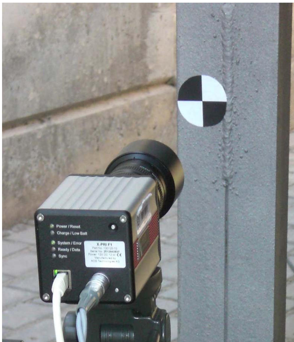
FIGURE 2 The high speed camera pointing to the target. The accelerometer is hidden at the left part of the column. 430x497mm (72 x 72 DPI)
