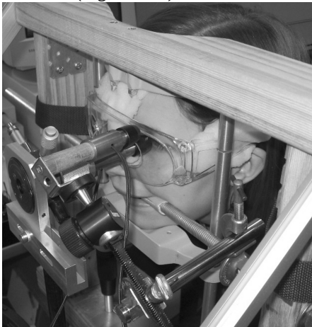
Fig. 1. The measurement setup for examination of longitudinal corneal apex displacement and antero-posterior head displacements (Experiment I). Simultaneously the ECG signal was registered. The subject is placed in the rigid headrest with a bite bar. Head movement is represented by the displacements of protective glasses worn by the examined subject.
