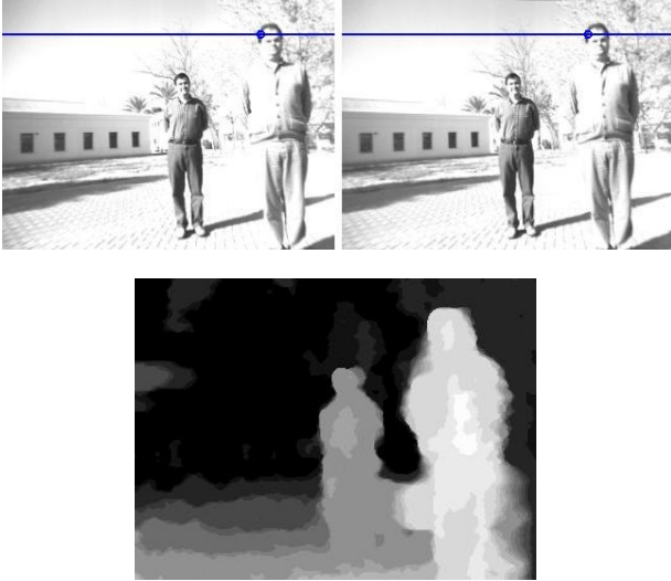
Figure 1. A stereo par showing an epipolar line (above). Image of disparity (below)
