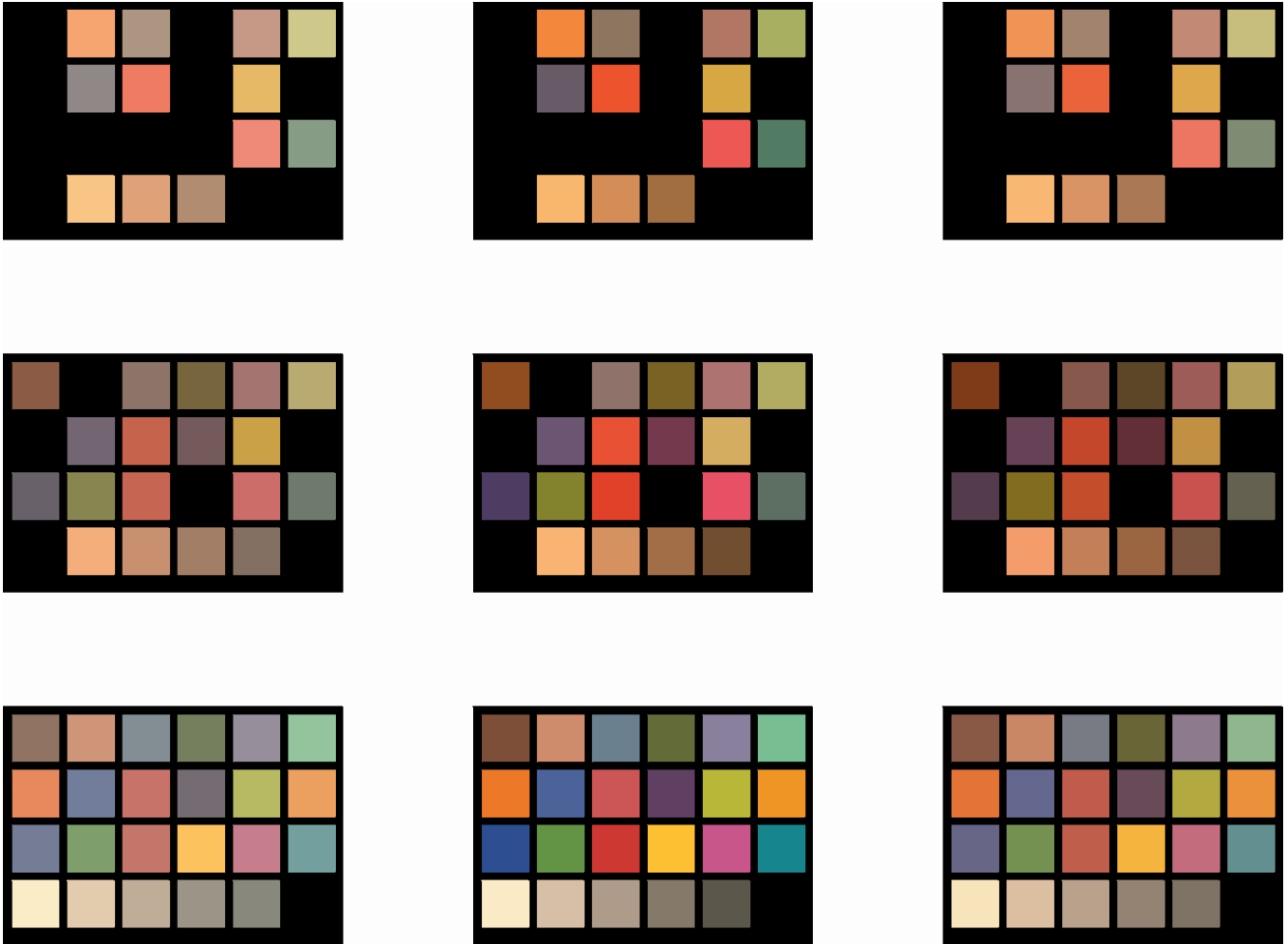
Color Plate 5. SRGB simulation of the ColorChecker chart captured by our color device under three light sources (top: incandescent lamp with N = 4 ; center: metal halide lamp with N = 5.6 ; bottom: fluorescent daylight lamp with N = 5.6 ). Left: raw reproduction model; center: original CIE-XYZ encoding; right: corrected reproduction model. (Notice that the original reproduction level of these colors may have undergone alterations even though the color management algorithms have been performed correctly.) ( Francisco Martínez-Verdú, et al , pp.279–295).
