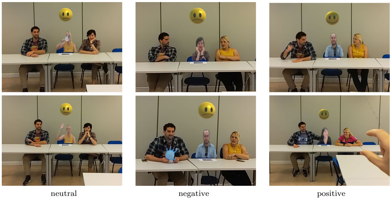
Fig. 5 Examples of visualizations obtained from the HoloLens 2 viewer with the proposed cyberpresence system running in the first test. Here, correct person segmentation and emotion classification are shown in each case
