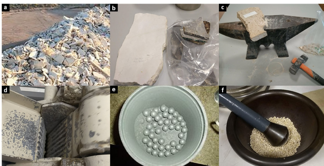
Figure 1. (a) Waste area of a marble company. (b) Waste collected from Ivory Cream and Imperial Brown. (c) Anvil and hammer. (d) Jaw crusher. (e) Ball mill. (f) Pestle and mortar.
