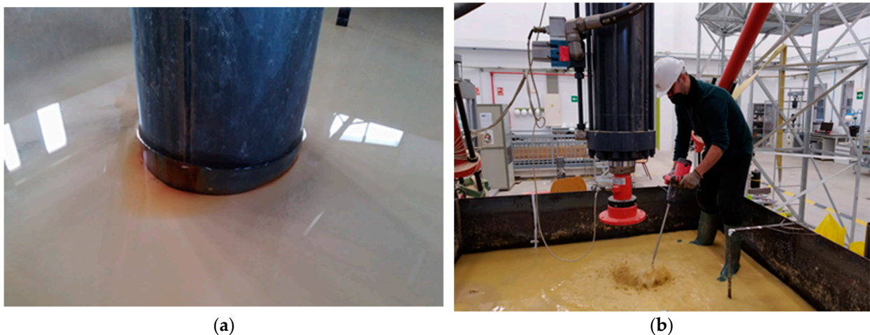
Figure 3. Phases of project: (a) testing a pile of 80 mm in submerged conditions; (b) sand decompressing.
