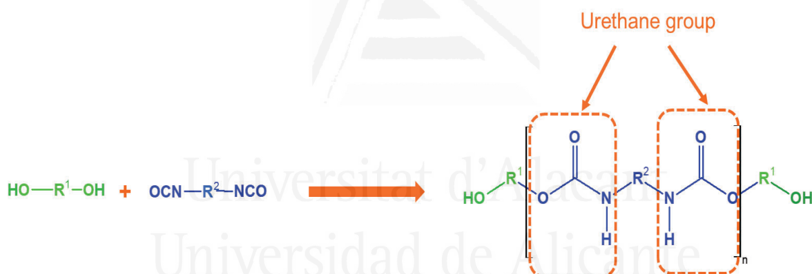
Figure 1.1. Basic reaction of the synthesis of the polyurethanes.
