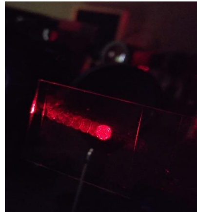
Fig. 3. Waveguide recorded on photopolymer.
