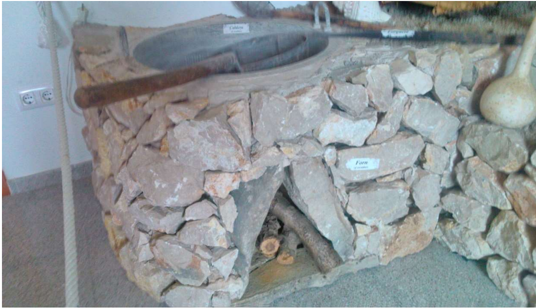
Figure 9. Stone oven (Forn) to make raisins. Inside the boiler (Caldera) the water is boiled with an alkaline plant and the grapes are introduced through a strainer (Cassa) to be treated. Ethnological Museum, Tàrbena.
