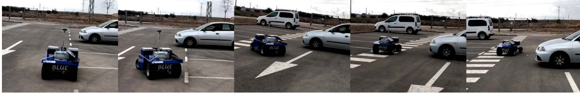
Fig. 12. Obstacle avoidance experiments: Example of car avoidance in an image sequence. The vehicle circulates in a straight-line way and modifies its trajectory when a car crosses its path.
