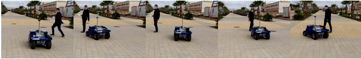
Fig. 11. Obstacle avoidance experiments: Example of pedestrian avoidance in an image sequence. A pedestrian crosses the vehicle trajectory twice (images 2 and 4 from left to right). In both cases, the vehicle avoids this dynamic obstacle by doing rear maneuvering.
