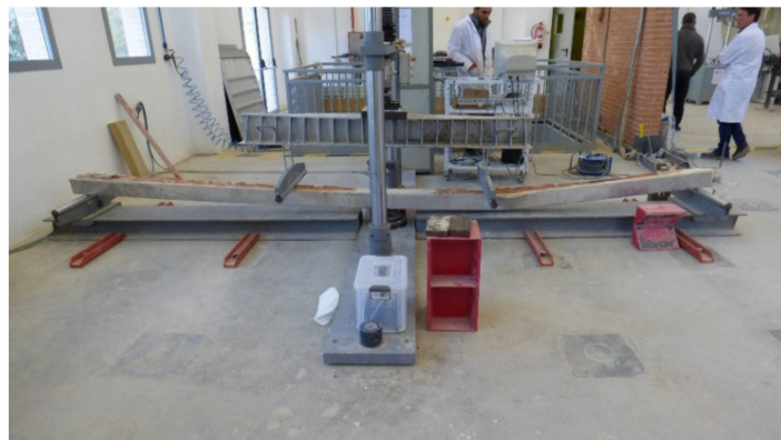
Figure 15. Prosthesis breakage test set-up.
