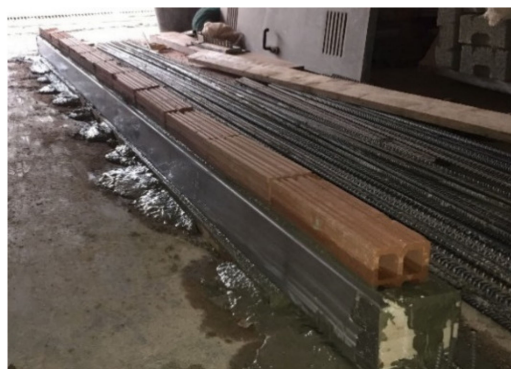
Figure 18. Specimen for the flexural test. Clay joist violin reinforced with a stainless-steel prosthesis.
