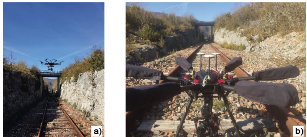
Figure 6. UAV DJI Matrice 600 Pro during flight (a) and detail of UAV (b).
