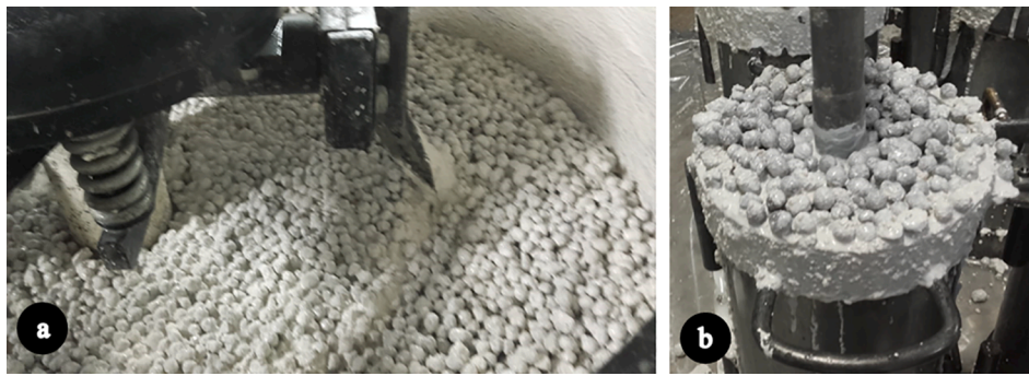
Fig. 6. a) Excessive fluctuation of lightweight aggregates in the mixer. It is observed that the aggregates on the surface are enveloped only by a thin layer of cement paste. b) Loss of lightweight aggregates during vibration (high vibration times).
