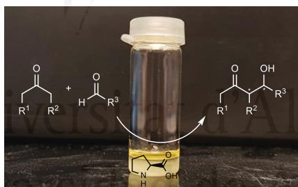
Figure 27. Eutectogel for catalytic application in the enantioselective aldol reaction.
