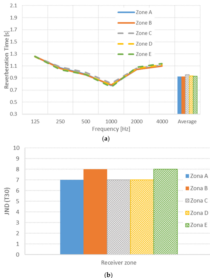
Figure 9. Reverberation time (a) and JND (b) obtained for the auditorium, when the variable acoustic solution provides maximum absorption, by zones (configuration A).
